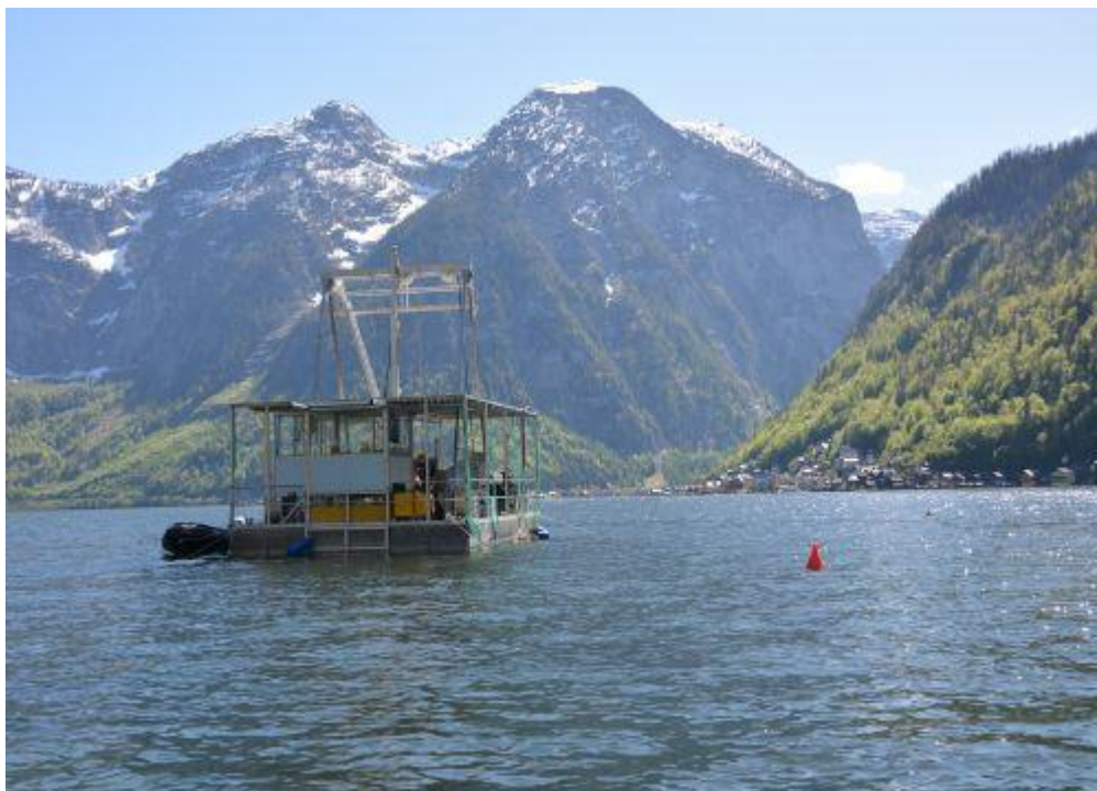
Figure 9: Coring lake Hallstatt with the Hipercore coring device. Image credit: Reschreiter/NHM Wien
