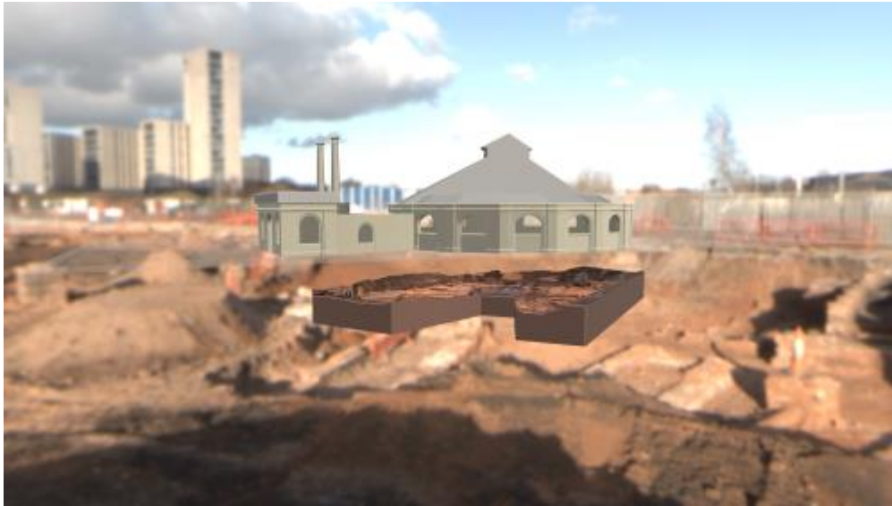
Figure 4: 3D modelled representation of the Railway Roundhouse at Curzon Street from original architectural drawings (CZNST/53; CZNST/54 and plans for the remodelled roof CZNST/61) using Blender to develop 3D models of the two roof forms.
