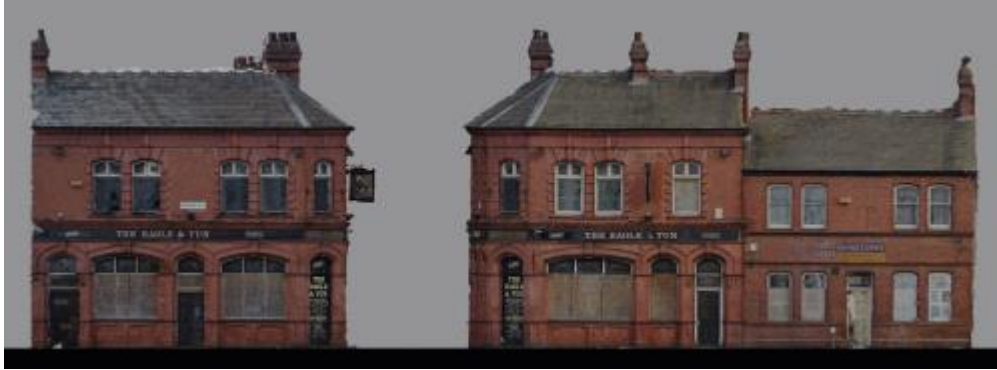
Figure 8: Reconstructed 3D model from scaled SFM photogrammetry of the Eagle and Tun public house captured prior to demolition and shown in two orthographic projections
