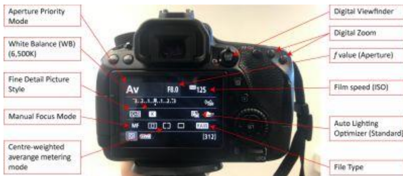
Figure 12: Info screen on the Canon EOS 80D showing the settings used. ©Mónica Palmero Fernández.
