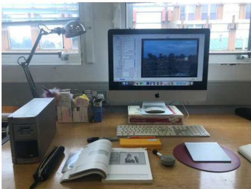
Figure 3: Workstation set-up with Nikon CoolScan IV ED and iMac computer with macOS High Sierra 10.13.4. This computer was used to test the Nikon scanner using VueScan 9 x64 (9.6.38) and SilverFast 8.8 software ©Mónica Palmero Fernández.
