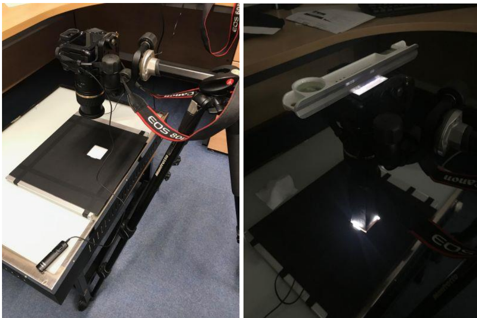
Figure 6: Final set up for scanning, showing the custom-made black cardboard slide holder attached to the LightPad to block out excess light (a) and the process of levelling the camera to avoid distortion and out-of-focus areas (b) ©Mónica Palmero Fernández.
