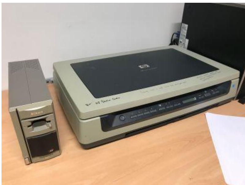
Figure 2: The two scanners tested for the project: Nikon Coolscan IV ED slide/film scanner (left) and HP Scanjet 8300 flatbed scanner (right). Both offered high resolution (2900 dpi and 4800x4800 dpi hardware, respectively), but seemed to struggle with the complexity of Kodachrome colour reversal film ©Mónica Palmero Fernández.
