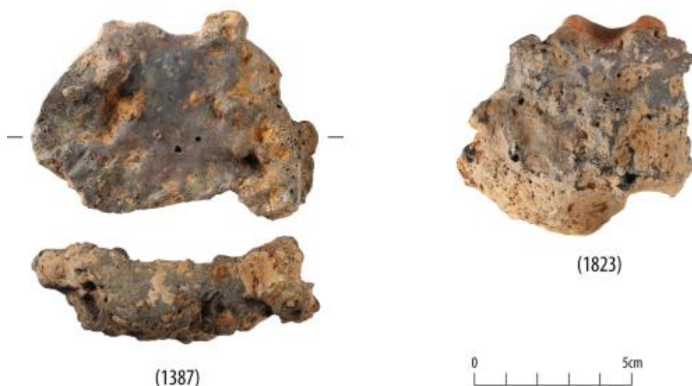
Figure 35: Industrial waste - smithing hearth bottoms from 1387 and 1826. Image credit: Headland Archaeology (UK)
